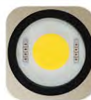
COB LED to provide 15000 lumens
